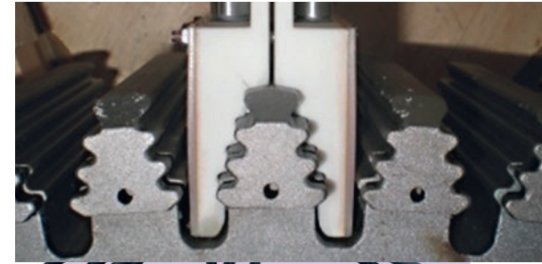
Inspection of the dowel tails of a gas turbine
